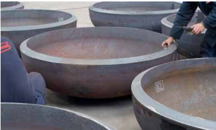
TYPE: 2:1 ELLIPSOIDAL HOT HOT FORMED OUTSIDE DIAMETER :1900 MM THICKNESS: 80 MM MATERIAL: SA 516 GR 70 N FOR PRESSURE VESSEL
