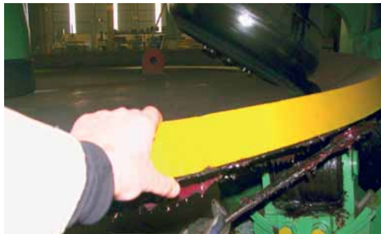
TYPE: FLAT HEAD OUTSIDE DIAMETER : 3100 MM THICKNESS: 75 MM MATERIAL: SA 516 GR 70 N LADLE FOR STEEL INDUSTRY
