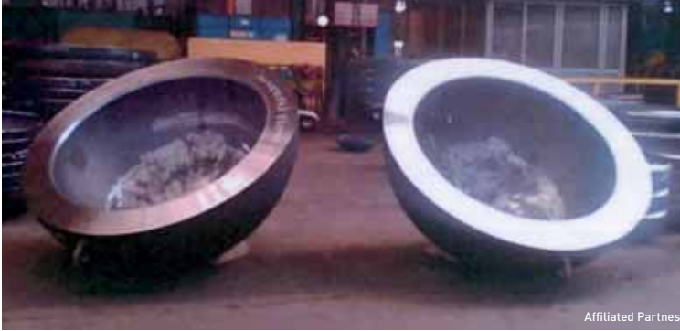
TYPE: HEMISPHERICAL HOT FORMED OUTSIDE DIAMETER :1475 MM THICKNESS: 230 MM MATERIAL: SPECIAL ALLOY FOR NUCLEAR REACTORS
