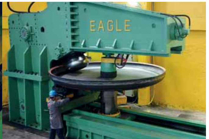
TYPE: FLAT HEAD OUTSIDE DIAMETER : 3100 MM THICKNESS: 75 MM MATERIAL: SA 516 GR 70 N LADLE FOR STEEL INDUSTRY
