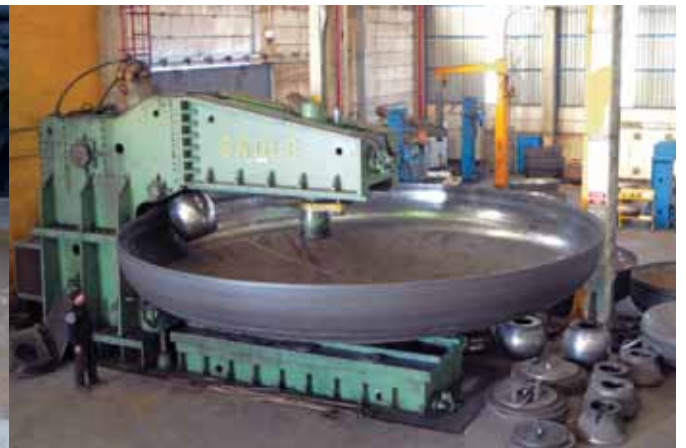
TYPE: TORI-SPHERICAL COLD FORMED OUTSIDE DIAMETER : 8000 MM THICKNESS: 50 MM MATERIAL: SA 516 GR 70 N FOR PRESSURE VESSEL
