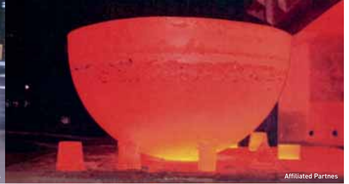
TYPE: HEMISPHERICAL HOT FORMED OUTSIDE DIAMETER :3100 MM THICKNESS: 250 MM MATERIAL: SPECIAL ALLOY FOR NUCLEAR REACTORS
